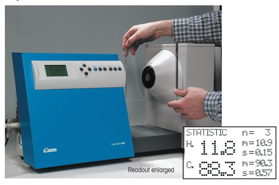
**haze-gard plus** is a laboratory instrument to objectively evaluate total appearance of transparent products. The optical properties of films and packaging material, clear and translucent specimens, and raw materials for paint and plastics can be differentiated by using the following measurement values: • Total transmittance • Haze • Clarity
